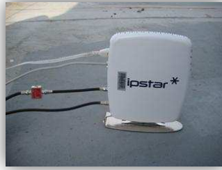
Figure 47: How Tx external attenuator connected with Sat Tx of IDU
