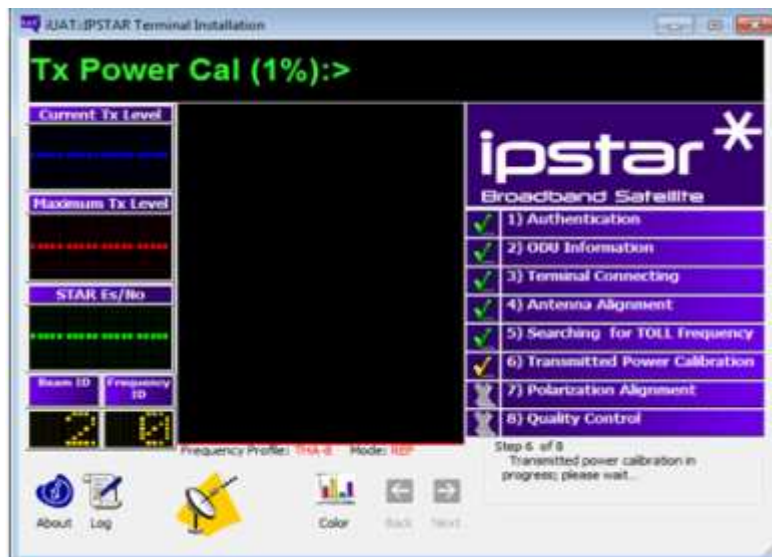
Figure 32: iUAT program is calibrating the transmitted power
