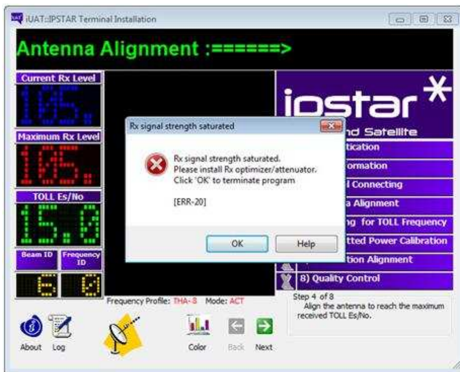
Figure 43: Rx signal strength saturated [ERR-20] message
