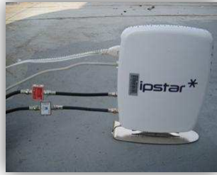
Figure 44: Inserting Rx external attenuator between Sat Rx port of IDU and LNB
